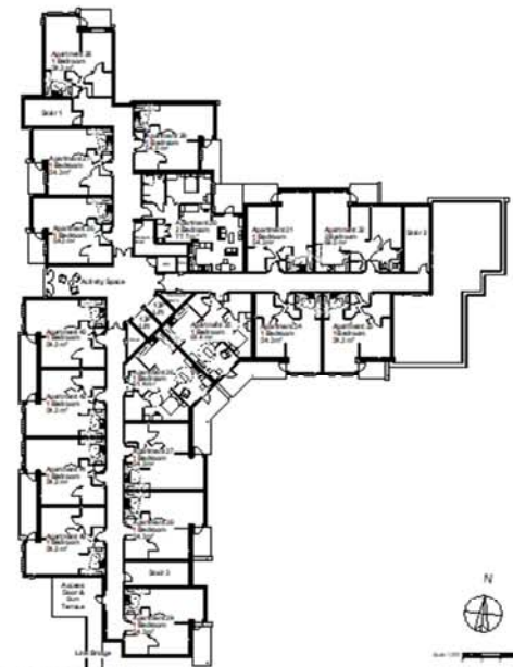
FIRST FLOOR PLAN
